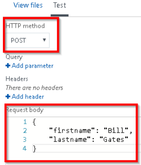
Figure 1.8: Testing the HTTP trigger with input data
