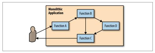
Figure II-1. A monolithic service with all functions in a single container
