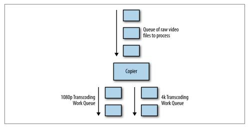
Figure 11-2. The copier batch pattern for transcoding
