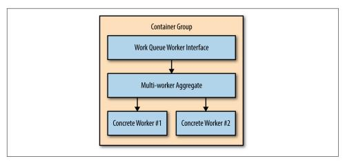
Figure 10-5. The multi-worker aggregator pattern as a group of containers
