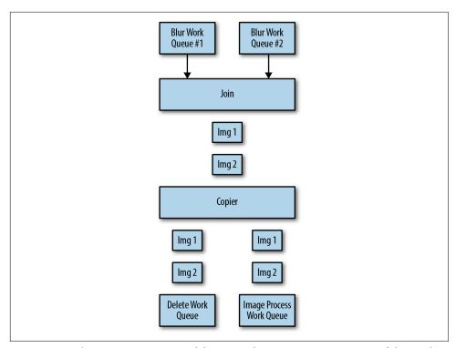
Figure 12-4. The output join, copier, deletion, and image recognition parts of the pipeline
