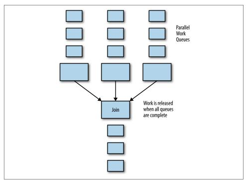
Figure 12-2. The join pattern for batch processing
