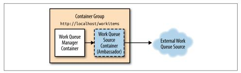
Figure 10-2. The same work queue as shown in Figure 10-1, but this time using reusable containers. The reusable system containers are shown in white while the user-supplied container is shown is grey/blue.
